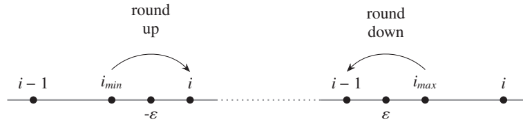
Figure 6.8 Approach for handling the case where the heater start/end does not align with the location of the nodes.
